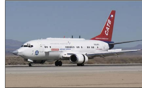
COTS Journal July 2014: Figure caption: Project Missouri demonstrations successfully implemented and tested two data links between an F-22 and the F-35 Cooperative Avionics Test Bed (CAT-B) (shown).
