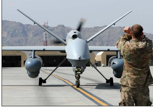
The Aviationist April 5, 2015: Photo Shows A U.S. reaper drone carrying "Gorgon Stare" wide area airborne Surveillance system pod in Afghanistan
